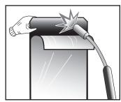
Peel back about 200mm of release liner from the trimmed end of the sleeve. Gently heat exposed adhesive.
