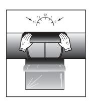
Position the heated adhesive on the pipe surface between the 10 and 2 o'clock position so that the sleeve overlaps onto the adjacent coating by 50mm minimum.
