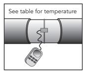
Measure the surface temperature to confirm that the correct value is achieved. An appropriate shelter may be used in wet or windy conditions.
