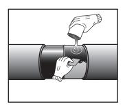
Mixing and application Instructions are provided with the Premier Epoxy pack. Apply the mixed Premier Epoxy to the steel surface at a uniform thickness of 100 microns (minimum). In a single operation, the primer is applied to the full width of the joint and at least 50mm onto the adjacent pipeline coating. The remaining stages of application are carried out whilst the primer is still
