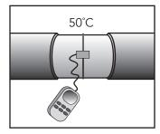
Heat the steel surface to 50°C prior to blasting to avoid formation of condensation and prevent flash rusting.
