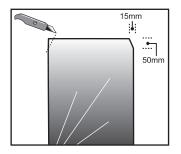
At the end of the sleeve that will form the underlap, use a knife to trim the corners (15mm x 50mm) as shown.
