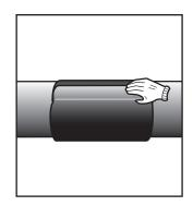
Heat the closure patch and attach it centrally to the overlapping end of the sleeve. With gloved hand press down firmly into place.
