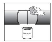
Thoroughly clean the area of the welded joint and the adjacent coating.
