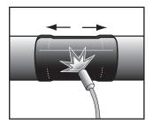
Use a blue flame and a continuous sweeping motion. Heat the sleeve starting from the centre and then heat around the pipe circumferentially.
