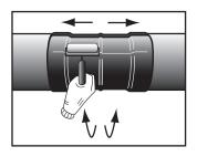
Whilst the sleeve remains soft, use a hand roller to remove any entrapped air. Start at the underside of pipe and work towards the crown.
