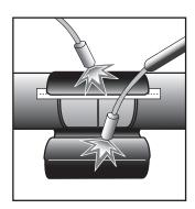
Completely remove the remaining release liner. Loosely wrap the sleeve around the pipe. Gently heat the sleeve at the underlap and the adhesive side of the overlap.
