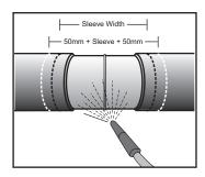
Standards Organization ISO 8501-1 Sa 2½. An abrasive blast profile of 50 microns minimum is required. Clean the area of the welded joint and the adjacent coating. The area cleaned shall extend at least 100mm on to the adjacent coating.
