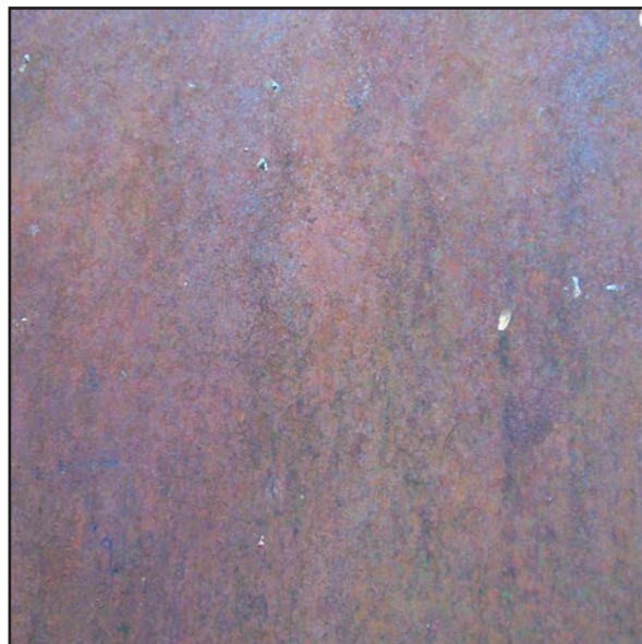
Example image of an acceptable level of surface preparation.
