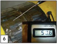
Measure the preheating temperature with an appropriate temperature sensor.
