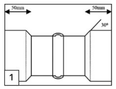
Ensure the Heat Shrink Sleeve is wide enough to overlap the factory coating by 50 mm minimum. Bevel the edges of the factory coating with a rasp with semi-circular blade to an angle of 30°.
