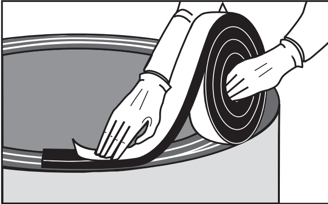
Fig 3. Apply Premstrip TM across the groove and remove the interleaving.
